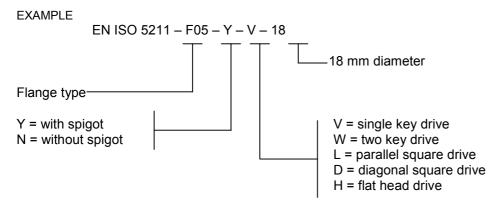
EN ISO 5211 - F05 - Y - V - 18, identifies a part-turn valve actuator attachment in accordance with this standard, with F05 flange type, spigot and single key drive with 18 mm diameter.
